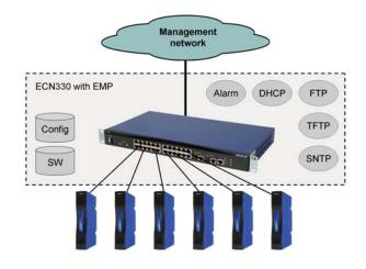
In this way, there is only one management interface and one static IP address. For provisioning, the EMP is managed via standard MIBs, and for system maintenance via EDA SNMP MIBs. All SW images and configurations are stored in local non-volatile memory to secure full operation, even if access to the management system is unavailable.
